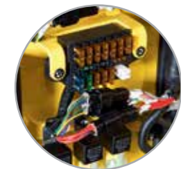
Concentrated Fuse Box for Easy Inspection
