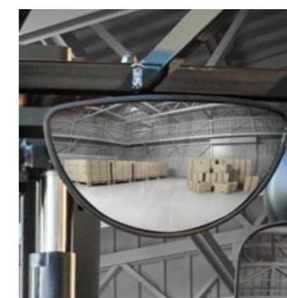
Panoramic mirror The panoramic mirror expands the driver's view when reversing the machine.
