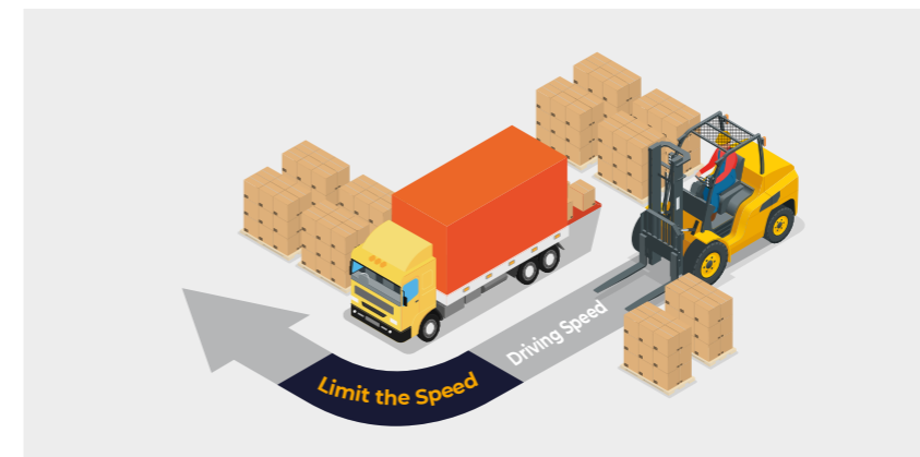
Curve Control The Curve Control system limits travel speed based on the turning radius, ensuring that turn manoeuvres are smooth and precise.
