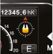
Speed adaptive steering The steering angle sensor displays the machine's travel direction on the screen. The speed of the truck is reduced as the steering angle increases.
