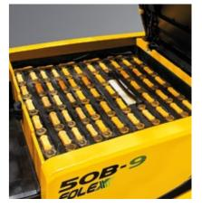
Easy battery maintenance The battery cover opens fully to improve access. It is equipped with locking gas
