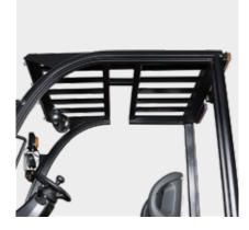
Strong overhead guard Exceeding EEC and ANSI requirements, the overhead guard offers excellent protection without restricting visibility.
