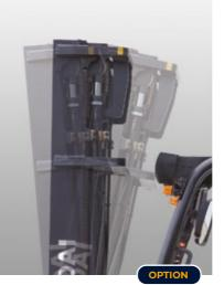
Auto fork levelling system This feature ensures that mast tilting stops smoothly when the forks are in a level position, improving both productivity and safety.
