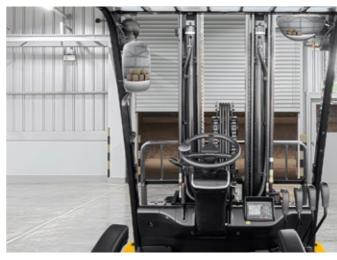
The 9 Series forklifts feature an antiroll-back system that prevents them from rolling back on a slope and offers exceptional drive-off capabilities.
