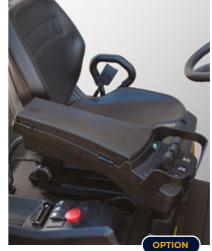
Fingertip control lever and adiustable armrests The electric control lever makes operation almost effortless. The ergonomically designed armrests can be adjusted up and down and from front to back, to fit different body shapes and reduce fatigue.
