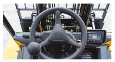
The steering wheel diameter has been reduced by 40 mm to minimise driver fatigue. A Danfoss 4th generation Orbitrol steering unit has been added to reduce noise and improve rotation.
