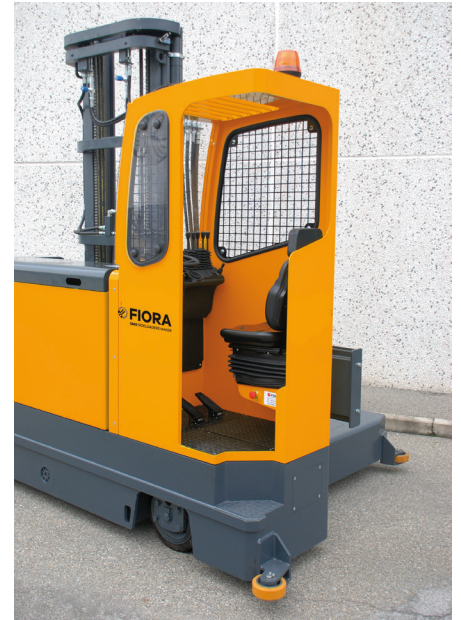
Side drive cabin , ergonomic and fully adjustable seat, lined in a sturdy hypoallergenic material. The 45% entrance makes the access in the cabin easy and safe even when the forklift is in the aisle.
