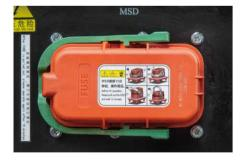
Both the battery and junction box have MSD maintenance switches to enable one-click power-down and safer maintenance.
