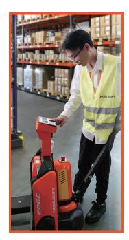
LCD digital numbers are upto 30mm in height, data can clearly be seen, there is a background light source, suitable for applications in dark environments.
