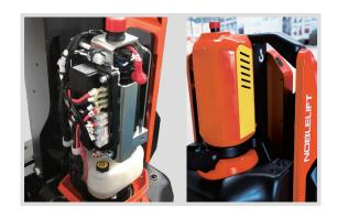
These trucks are equipped with CURTIS controllers, CAN-bus technology makes the diagnostic and troubleshooting easier.
