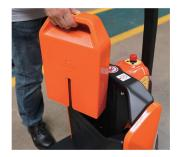
Light weight of the battery (max. 8kg) and the way of fast battery replacement allows even a female operator to double the work time within seconds. The light weight of the batteries can be achieved through use of li-ion battery type with high ratio of energy density to its self-weight.
