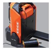
Socket on battery case for easy battery charging without necessity to take the battery out. The PTE15N SC reamins
